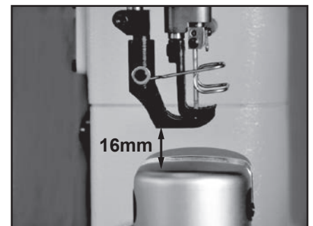
The clearance under the presser foot (16mm)
