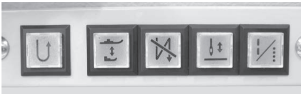
Simple setting for walking foot movement
