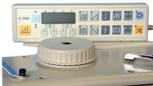
Simple setting for alternating presser foot movement
