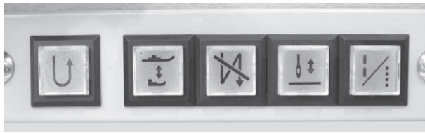
Simple setting for walking foot movement
